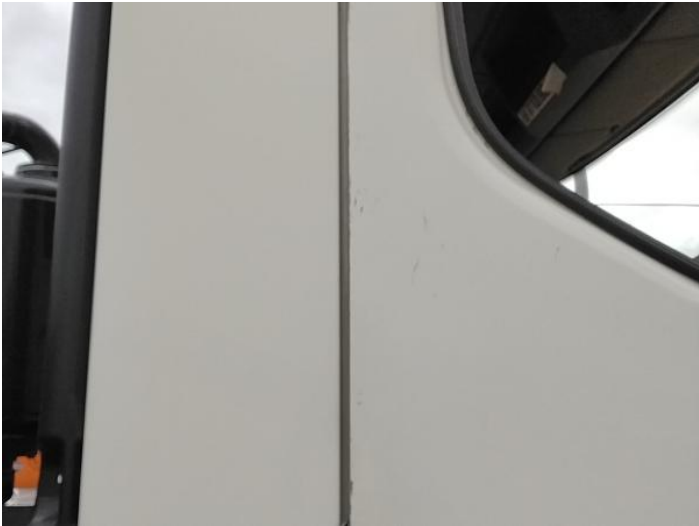
9: Door osf Chipped Edge Chip
